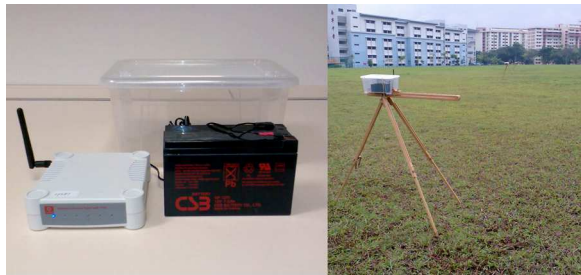
Figure 3: Wireless router and accessories used in the testbed. Left: One node is composed of one Compex WP54G router, one 12V rechargeable lead battery and one plastic container to protect the hardware from rain. Right: Actual deployment of the node in the test site.
